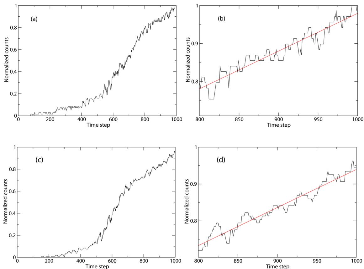
**Figure 1.** Cumulative histograms for the calculation of the first term for hydride (a) and deuteride (c) systems, normalized to unity integral. Fits of the linear region, from 800 to 1000 time steps (400 to 500 fs), are shown for hydride (b) and deuteride (d) systems. The slopes of these linear fits are the values for the first term of the rate calculation. Note that a time step corresponds to 1/2 fs.
